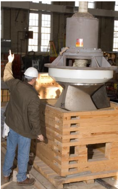
New pull-out assembly is delivered to job site after factory testing
